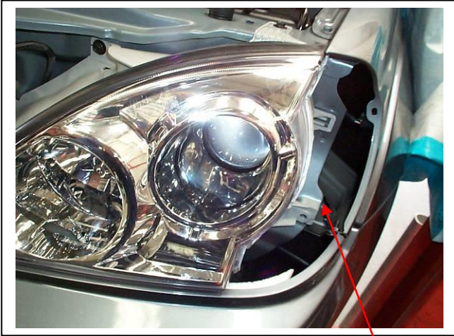
Figure 3 10mm Nut for bumper cover
