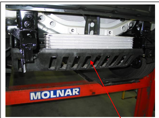
Figure 5 Remove plastic under guard
