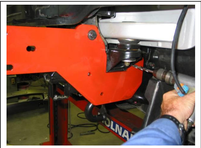
Figure 11 Shown drilling rear hole on passenger side chassis
